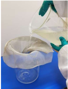
Filtration of Recovery Solution (comprising of recovered Resin)
