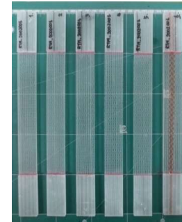
Composite Specimens from Fresh Fabrics (Before & After Test)
